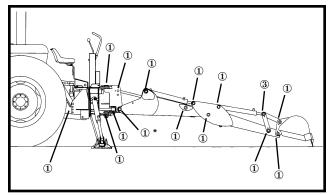
Figure 7 - Lubrication Points for Model 765H
